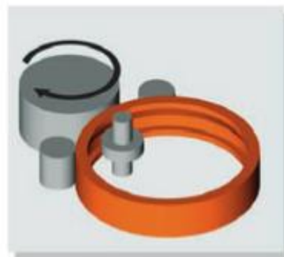
(b) Radial incremental ring rolling
