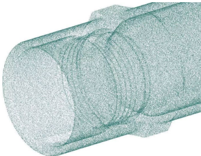
Obr.4 Mracho bodov získané 3D skenerom (Cadcaml, 2020)
